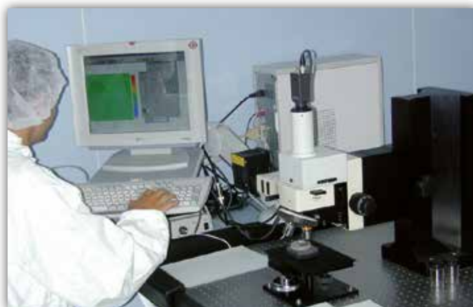
Quality control: microroughness measurement
