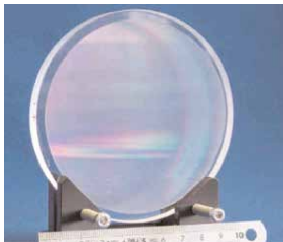
Example of a high efficiency IR transmission grating (GRISM) directly etched into an IR grade fused silica substrate
