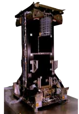
FUSE spectrograph with four aberration corrected holographic gratings, 5800 l/mm, 300x300 mm
