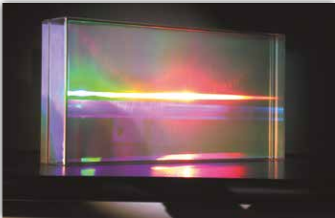
A 210 x 420 mm size Multi Layer Dielectric grating
