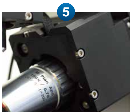
XYZ 物镜扫描器，将拉曼激光耦合到针尖尖端
