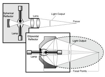
For the same bulb, the OBB PowerArc<sup>™</sup> delivers 5 to 6 times more light to the secondary focus! That means that an OBB PowerArc<sup>™</sup> lamp housing with a 75 watt xenon lamp provides the equivalent optical power of a 450 watt xenon lamp in an old style vertical lamp housing. And it does so with greater power density due to a smaller focal spot, and at a small fraction of the cost of a big old 450 watt illuminator.
